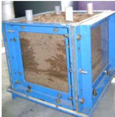
Fig. 2 Tank set up after the grout
