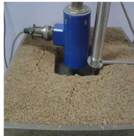
Fig. 3 Load cell with LVDT
