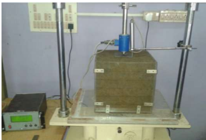
Fig. 2 Plate Load Test setup
